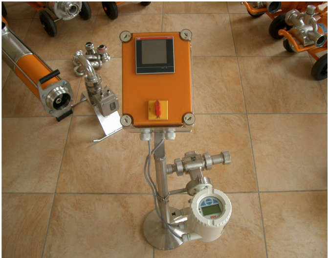
Fig. 13: Components of a batch dosing system with electromagnetic flowmeter and compact controller AC500eco
