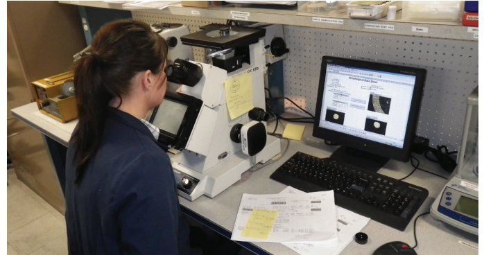
A lab service technician uses a metallurgical microscope to examine the microstructure of the metallic components in Watlow's mineral insulated metal sheathed cable, XACTPAK.
