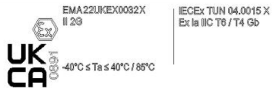
Figure 22: Ex marking (example, UKEX)
