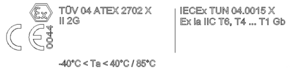
Figure 21: Ex marking (example, ATEX / IECEx)
