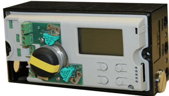
Figure 7: Open TZIDC with a view of the operating panel
