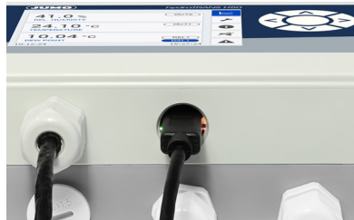
Fig. 39 Plugged USB cable and LED indication
