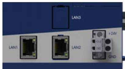
Fig. 3-1 LAN interfaces of the JUMO variTRON 500 (LAN1 as a standard feature, LAN2 as an optional extra)
