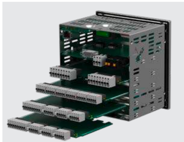
Example of possible measuring card placement
