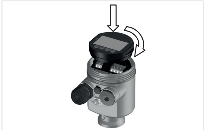
Fig. 53: Installing the display and adjustment module in the electronics compartment of the single chamber housing
