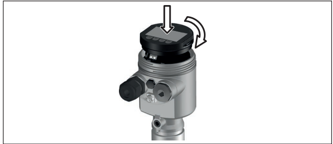
Fig. 17: Installing the display and adjustment module in the electronics compartment of the single chamber housing
