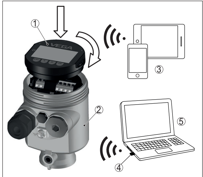
Fig. 1: Wireless connection to standard operating devices
