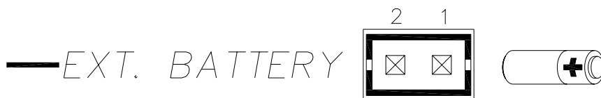
Figure 16 External battery connector for GF_VEDO HL terminals
