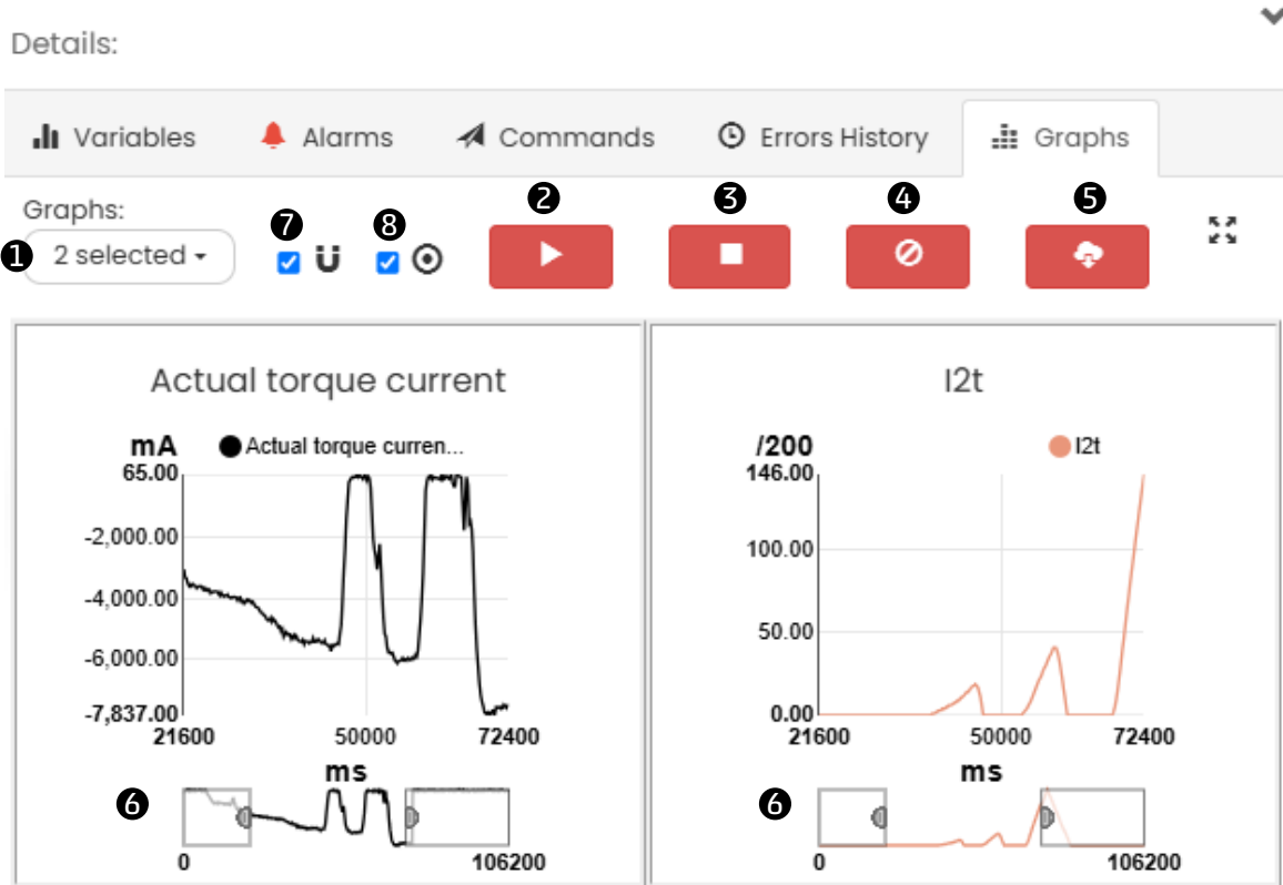
Figure 8.7: Section for graphing variables over time. In this example flag ⑦ is set, so Actual torque current and I2t are graphed over the same observation interval.
