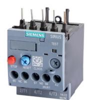
Overload relay 2.8...4.0 A size S00, class 10, for motor protection for mounting onto contactors main circuit: screw terminal AUX. circuit: screw terminal manual automatic reset
