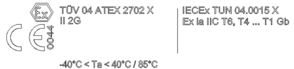
Figure 20: Ex marking (example, ATEX / IECEx)
